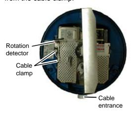
Antenna unit, cover removed, top view
